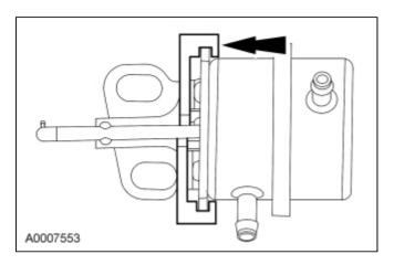
2. Align the actuator rod with the slot in the linkage, and rotate the <u>SC</u> bypass vacuum actuator into position.
